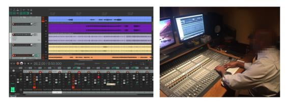
Figure 1: Left: A screenshot of the complex user interface of a Digital Audio Workstation showing 5 audio tracks above and the mixer console below; Right: A participant uses his control surface to perform audio production on his computer
